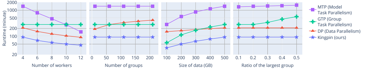
Figure 3: Analytical cost model-based plots for key scalability axes. Cost parameters are calibrated from real empirical runs presented later (Section 5) on Algebraic/LBFGS on Criteo dataset with grouping attribute Country. The dataset size is 488GB; Country has 18 groups; ratio of largest group, n_{max}/n , is 0.26. We set p = 4 workers. For each plot here, we vary one variable, while fixing all other workload properties.
